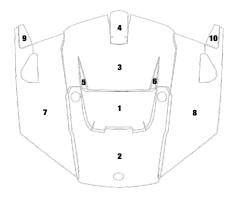
**Graphics Kit Install Order - Driver Side:** Install kit pieces in the order listed below starting with number 1. For aftermarket doors install door piece after step number 9. Repeat install procedure for the passenger side.
